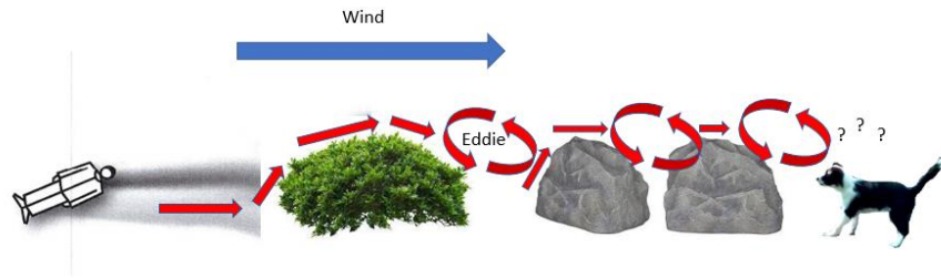
Figure 10: Forming of eddies and complications due to obstacles
